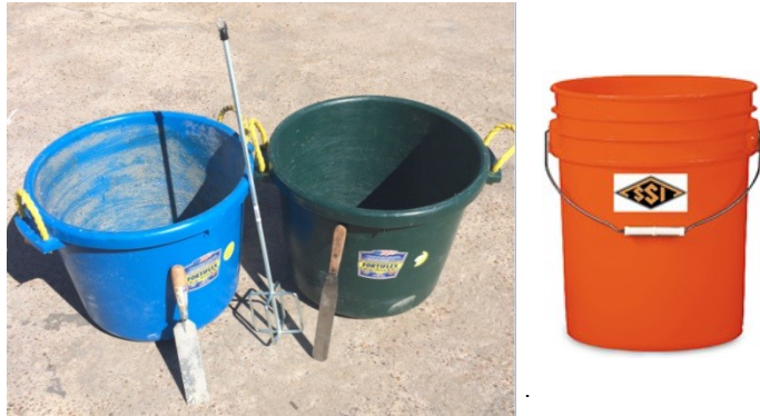
Mixing tools shown: Tub or bucket, mixing paddle, margin trowel, spatula to scrape cans.
