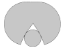
Figure 2. Enlarging Backer Rod by “Hot Dogging”
